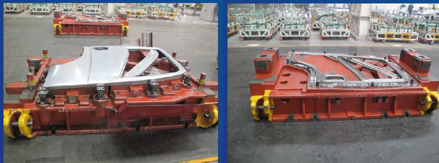
Flanging Die For Outside Door Panel
